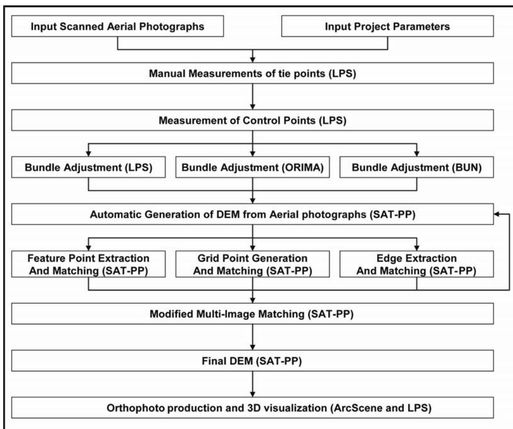
Fig. 3: Photogrammetric pipeline for DTM generation from aerial images.
