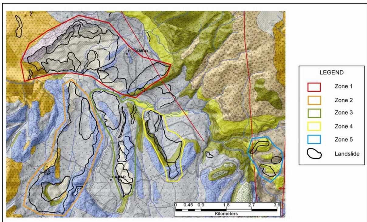
**Fig. 5:** Classification of the landslide processes using the derived DTM and orthophotos.
