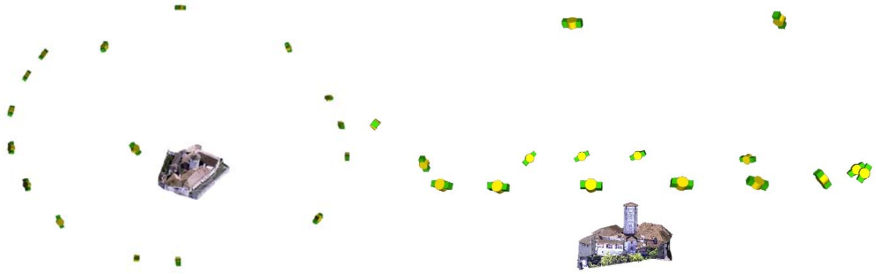
Figure 3. Recovered camera positions for the modeling of the overall castle from the 16 helicopter images.
