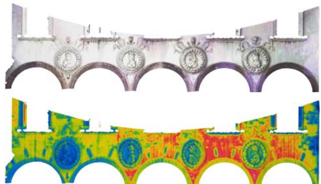
Figure 11. The range-based 3D model of the frontal part of the Loggia and the IR textured model.
