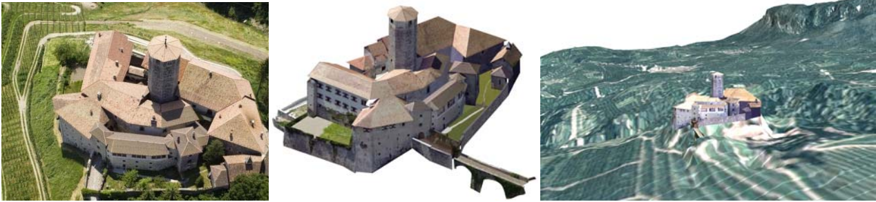
Figure 1: Helicopter view and produced 3D model of the ancient medieval castle of Valer, Trento (Italy) modeled using images. The surrounding landscape has been modeled with classical aerial images and then the castle integrated in the landscape model using GPS points [Voltolini et al., 2007].
