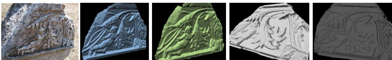
Figure 3: Stone example, modeled from 3 images: results respectively from NGATE, ATE, ARC 3D and SAT-PP.
