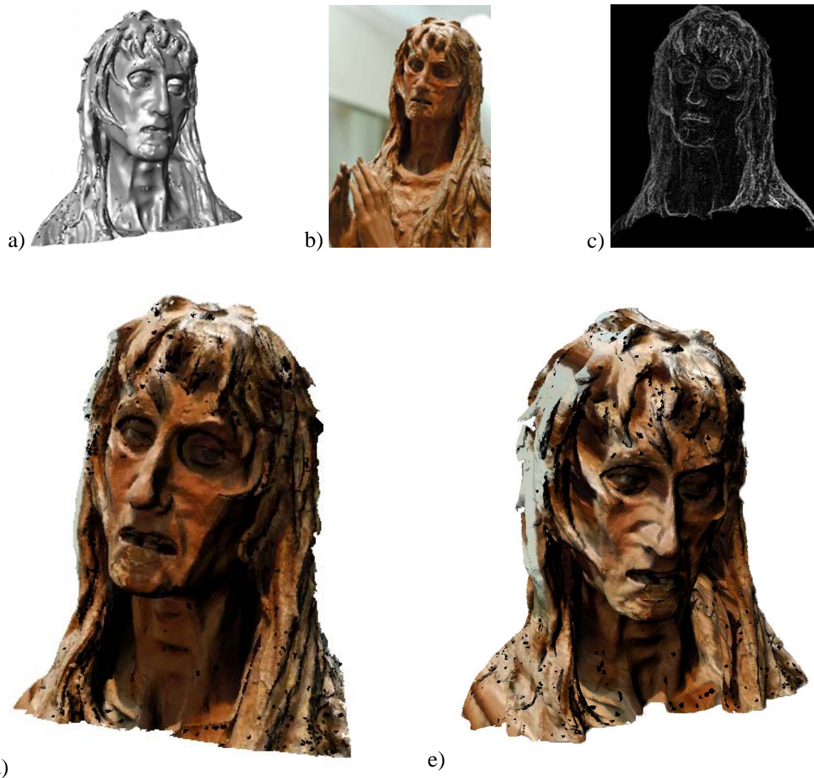
Figure 5: a) Screenshot of the geometric model of Maddalena's head [43]; b) An Internet image of the Donatello's sculpture; c) The computed depth map: please note the little amount of information shared with the texture image, which was nevertheless enough to accomplish a proper registration using the MMI criterion described in par. 3.1; d-e) Views of the textured 3D model obtained with the proposed method.
