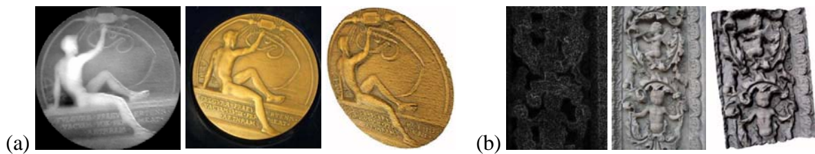
Figure 3: Two examples (coin and bass-relief) of the automated texturing method, showing respectively the generated depth map, the image to-be-mapped and the textured 3D model.
