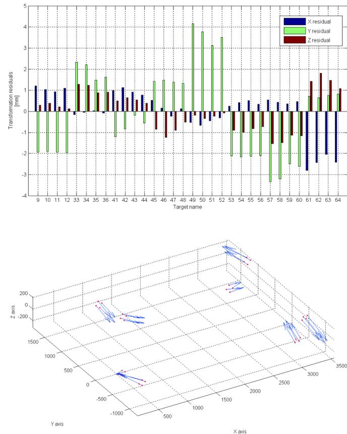
Figure 9. Residuals of the similarity transformation on the targets of the orientation devices.
