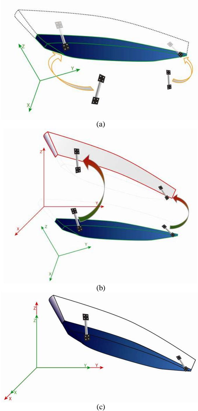
Figure 4 – Schematic procedure of the alignment of the two separate surveys above and below the waterline.
