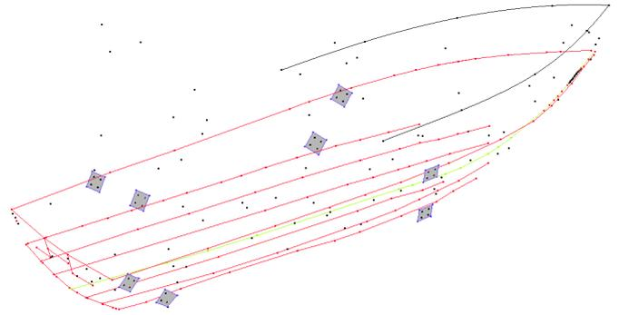
Figure 10. Feature lines and points measured in Photomodeler after the union of the two photogrammetric surveys.
