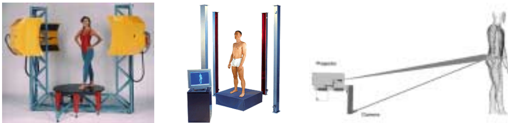
Figure 1: Two examples of 3D body scanner: Cyberware [8] (left) and Vitronics Vitus [25] (center). The triangulation process between projector camera and target subject.
