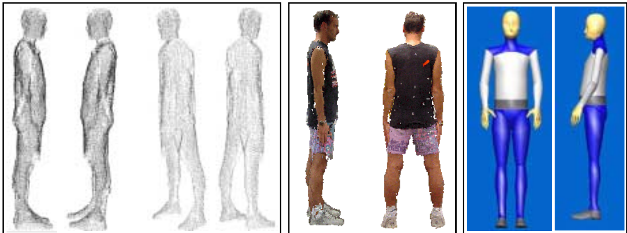
Figure 8: 3D point cloud of the human of figure 1 before and after filtering (left). Visualization of the 3D points with related pixel color (central). RAMSIS [18] human model which can be used to model the recovered 3D data (right)
