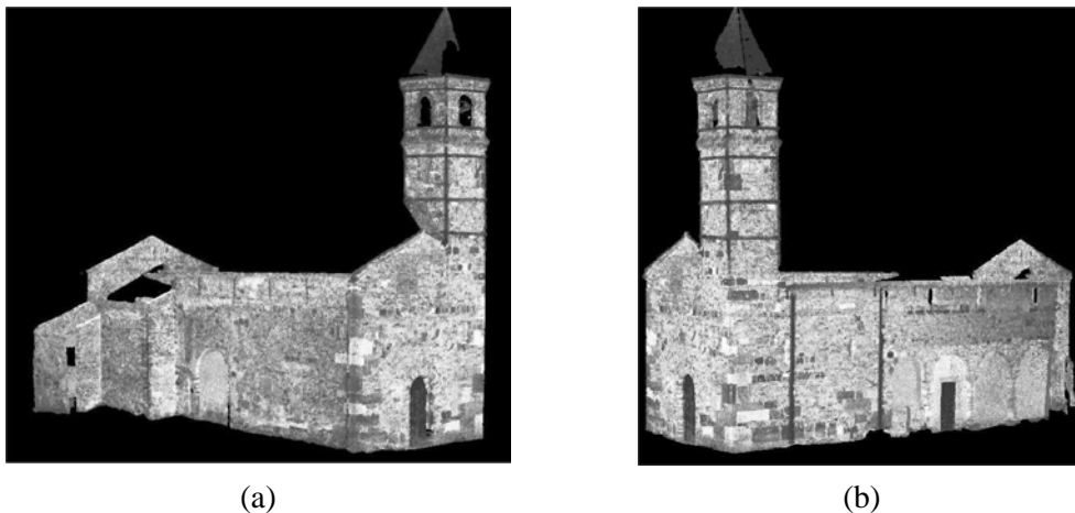
Figure 11: Two side views of the decimated 3D model of the church as point cloud.
