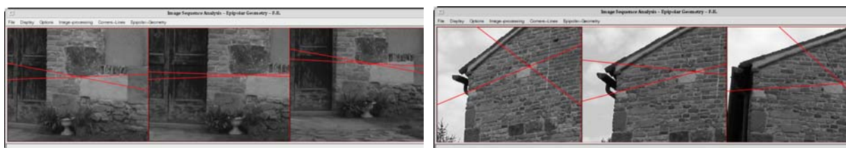
Figure 6: The epipolar geometry between image triplets recovered in photo-triangulation.
