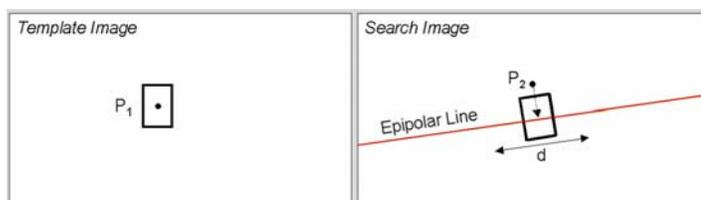
Figure 1: Stereo matching with search constraints.
