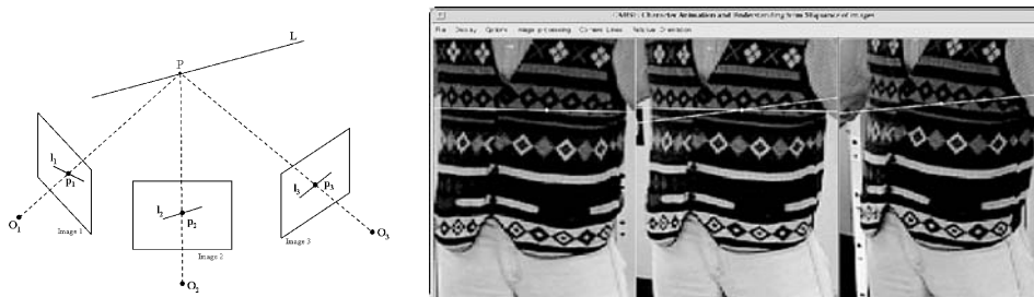
Fig. 4. Three views geometry: correspondences \mathbf{p}_i and \mathbf{l}_i corresponding to point P and line L (left). Relative orientation between triplet of images (right).
