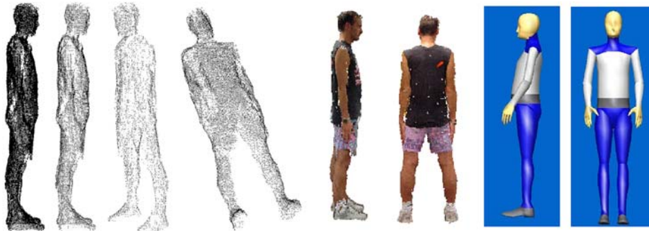
Fig. 9. 3-D point cloud of the human body imaged in Fig. 2: pre and after filtering results (ca. 20,000 points) and other views (left). Visualization of the recovered point cloud with pixel intensity (middle). RAMSIS [40] human model which can be used to model the recovered 3-D data (right).
