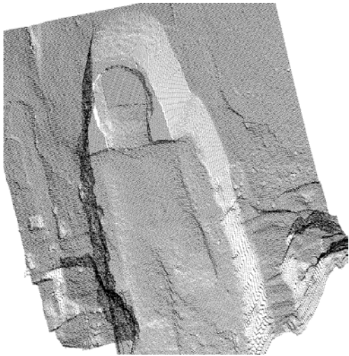
Figure 5: 3D point cloud generated with VirtuZo automatic matching on the metric images (ca 178 000 points).
