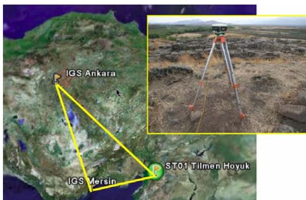
**Fig. 2. The reference point and its connection to the near GPS permanent stations.**
