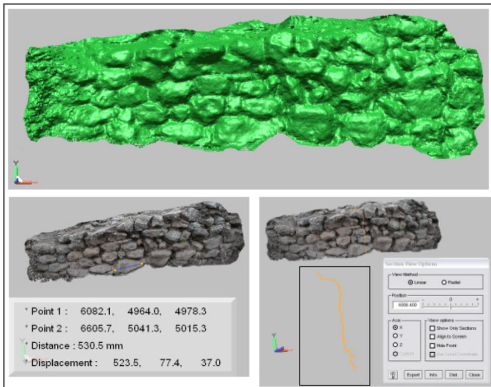
**Fig. 8. The 3D model of the wall and simple applications: distance measurements and sections.**
