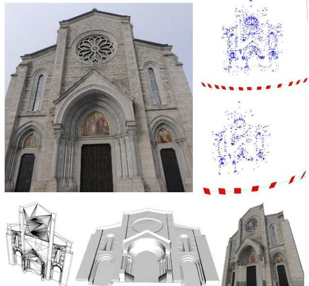
Fig. 5. A sanctuary façade and the camera poses with the sparse 3D point cloud (above). At the bottom the produced geometric 3D model of the church façade is shown.
