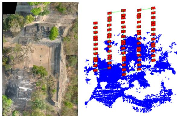
Fig. 8. A mosaic over the East Court (left) and the oriented image block composed of 70 UAV images.
