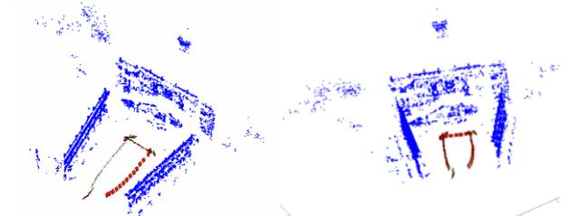
Fig. 6. The “Piazza del Campidoglio” sequence, made up of 52 images. The bundle adjustment derived a sparse point cloud of ca 11,800 3D points.
