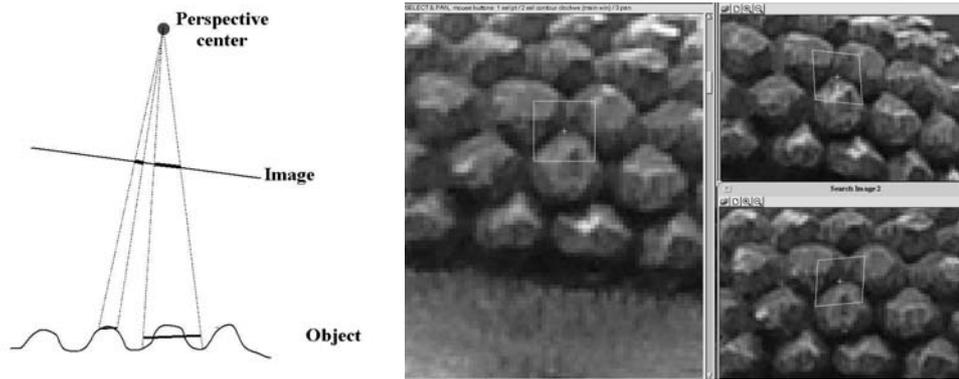
Figure 2. Patch definition in template least squares matching (left). Triplet of images where patches assumed to correspond to planar object surface patches where the assumption is not valid (right).
