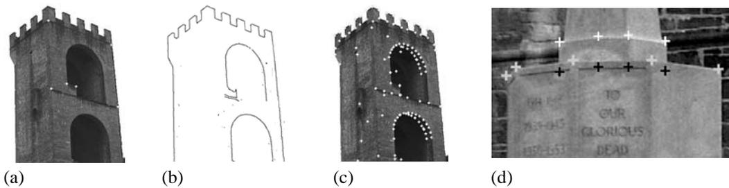
Figure 6. Automatic point extraction on arches (a). Constructing blocks (b). Seed points (c). Detected edge (d).
