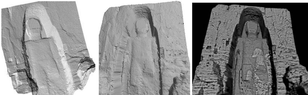
Figure 11. 3D model of the Great Buddha of Bamiyan (displayed as point cloud, shaded and textured model) generated with automated measurements. The automated matching procedure smoothed out all the small details of the folds present on the statue.
