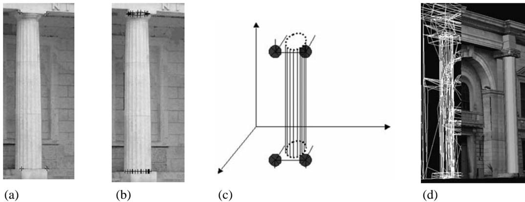
Figure 5. (a) Four seed points are extracted on the base and crown, (b and c) column points are added automatically, (d) column model.
