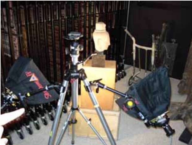
Fig.7. Illumination system used for the texture mapping.
