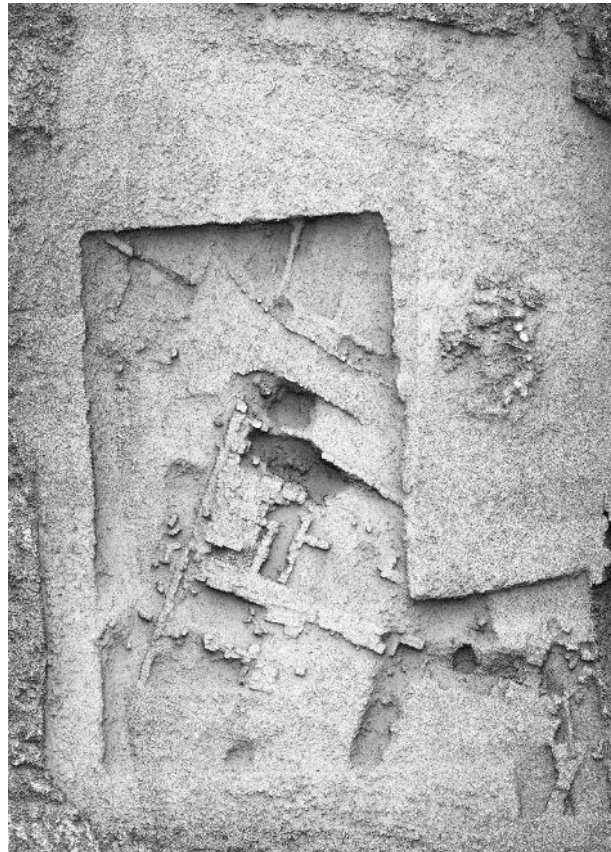
Figure 3: Micmac matching results with the UAV images over Veio, visualized in shaded mode.
