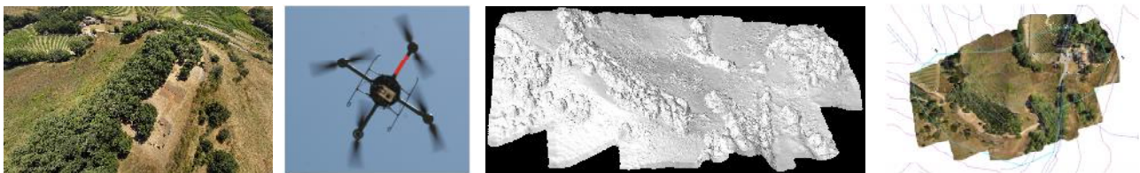
Figure 1: Example of scenes surveyed with a UAV system (Microdrone MD4-200) and photogrammetric results achieved from the acquired images: digital surface model, orthoimages and overlaid contours (archaeological area in Montalcino, Italy).
