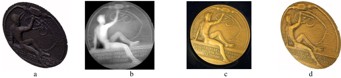
Figure.3 - In a) the textured model automatically generated is shown. In b) the computed depth map generated from the scanned 3D model, where the reliefs are clearly visible, varying from the dark (lower areas) to the white (upper areas), is displayed. Once the photo c) of the coin has been correctly registered with the map, it is possible to accomplish the texture mapping, leading to the model depicted in d).
