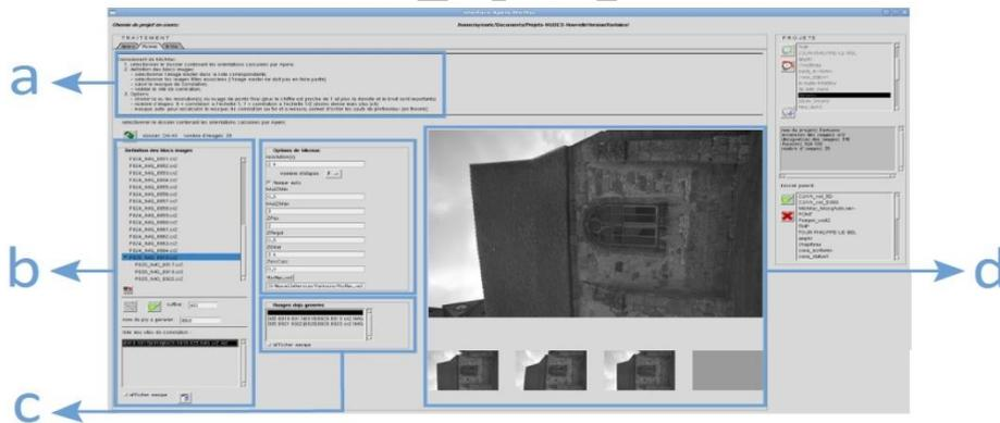
**Fig. 3.** GUI for the dense matching reconstruction step using MICMAC. (a): various explanations about point cloud generation; (b): the correlation tree, containing the list of all the available images; (c): the list of the previous point clouds generated within this project; (d): the current correlation images).
