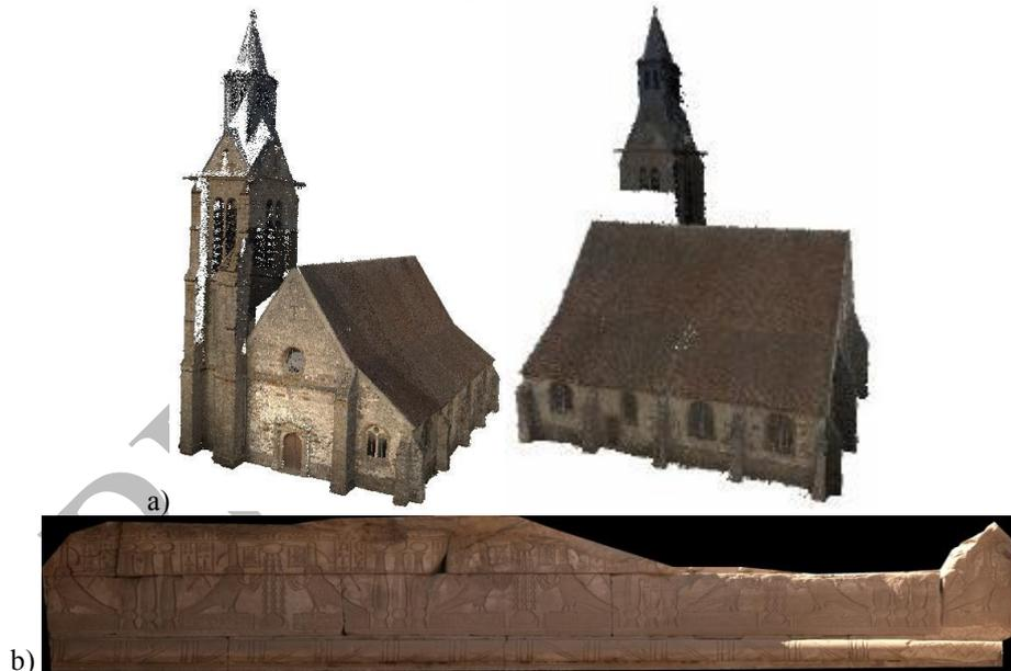
**Fig. 4.** Two examples of the results achievable using the developed image-based pipeline and GUI: a 3D point cloud of the Fontain Church, France (processing time: ca 3 hours) and an orthoimage of a bas-relief on the Dendera temple, Egypt (processing time: ca 1 hour).
