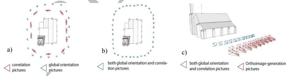
Fig. 2. Possible image networks for the surveying and modeling of a building.
