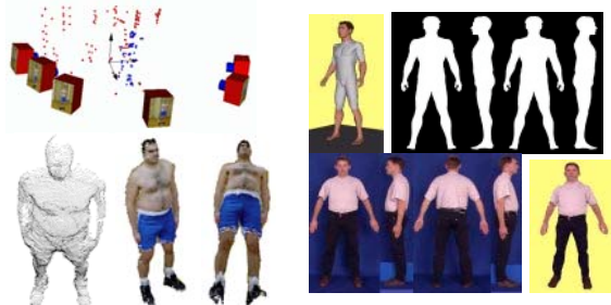
Figure 2: 3D model of static human recovered from a single camera image sequence (left) [24]. The process to recover 3D model using a silhouette extraction approach (right) [12].
