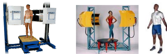
Figure 1: Example of body laser scanner. Vitus [32] (left) and Cyberware [7], with related 3D model (right).
