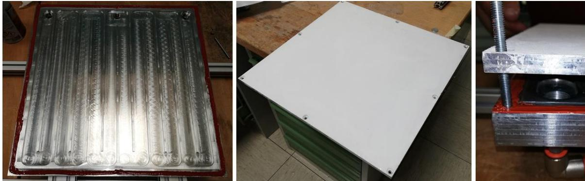
Fig. 7: Back support of the target with the water channel distribution (left), surface target coated with the painting (center), assembled phase (right).
