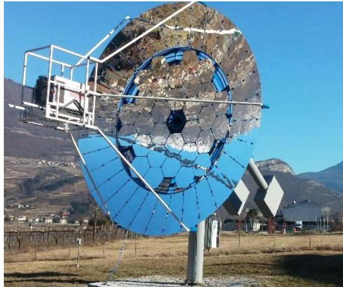
**Fig. 2: Front view of the system: the reflector presents spherically shaped hexagonal mirrors in the center and parabolic ones in the external ring.**
