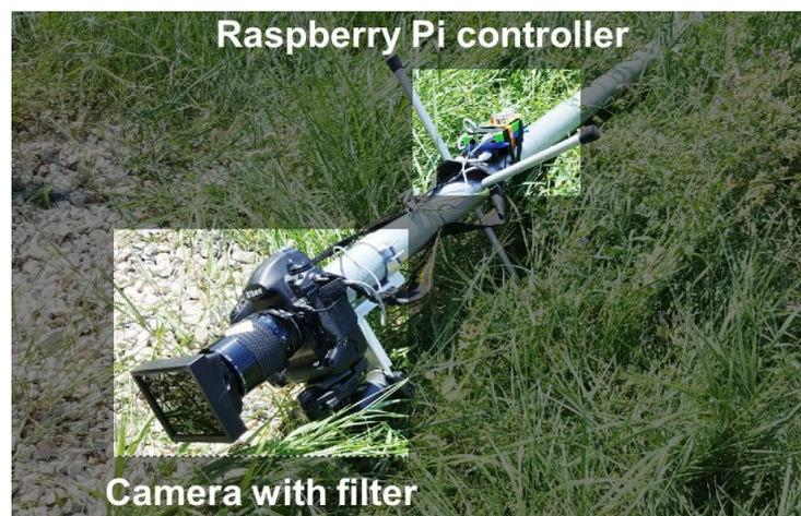
Fig. 8: Equipment used for the image acquisition fixed on the support.
